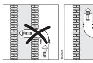
Never connect an exhaust hood to an active chimney, dryer vent, flue, or room venting ductwork. Seek professional advice before connecting an exhaust hood vent to an existing, inactive chimney or vent flue.
